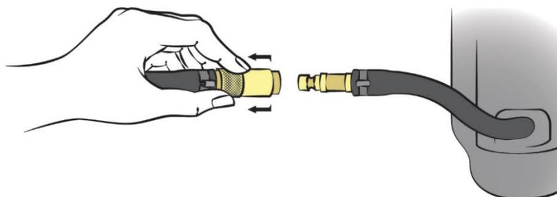
3. Release the barrel of the quick release fitting on the hose, so that it slides into the locked position.
