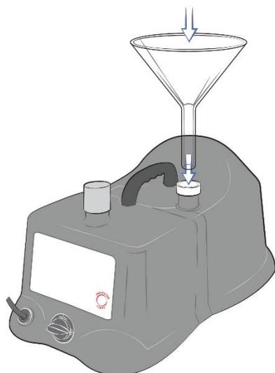
4. Carefully pour up to 3.5 litres of clean tap water into the steam generator.
