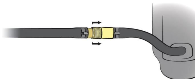
4. To check that the steam hose is securely connected, pull the hose. Ensure the hose is not kinked or restricted.
